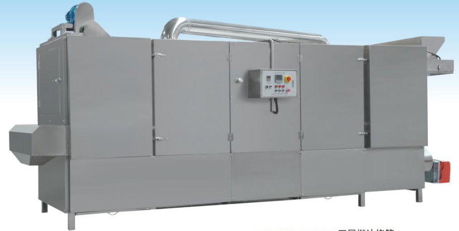
ZHKX-V-Y 五层燃油烤箱 5-Layer Fuel Oil Dryer
